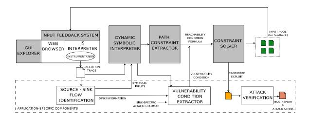
Figure 2.1: Architecture diagram for Kudzu. The components drawn in the dashed box perform functions specific to our application of finding client-side code injection. The remaining components are application-agnostic. Components shaded in light gray are the core contribution of this paper.
