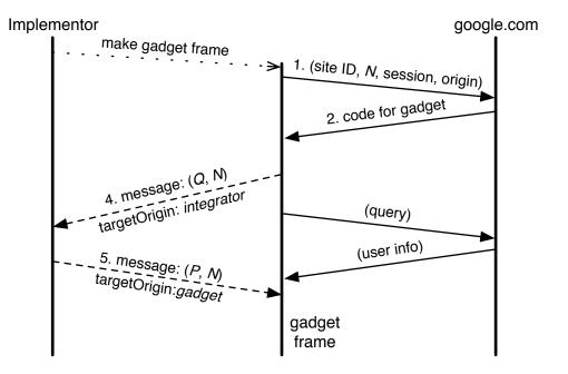
Figure 3.7: Google Friend Connect's gadget protocol: the nonce N is generated by the implementor. Message 4 is a query Q for parameters. The implementor responds with the parameters P in message 5.
