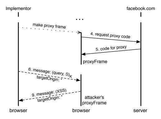
Figure 3.3: Integrity attack on Facebook Connect. Messages exchanged in the protocol. Note that midway through the protocol (after message 5), the request proxy is replaced by an attacker-controlled proxy.
