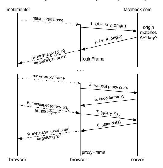
Figure 3.1: The Facebook Connect protocol. Ladder diagram of messages exchanged in the protocol. The dashed arrows represent client-side communication via postMessage and the solid arrows represent communication over HTTP. (query, S)  $_K$  represents a HMAC using the secret K. Frame hierarchy for the Facebook Connect protocol. In this example, the proxyFrame is inside the main implementor window.
